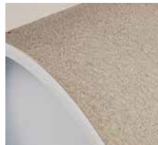
Cementgebonden speciale coating
